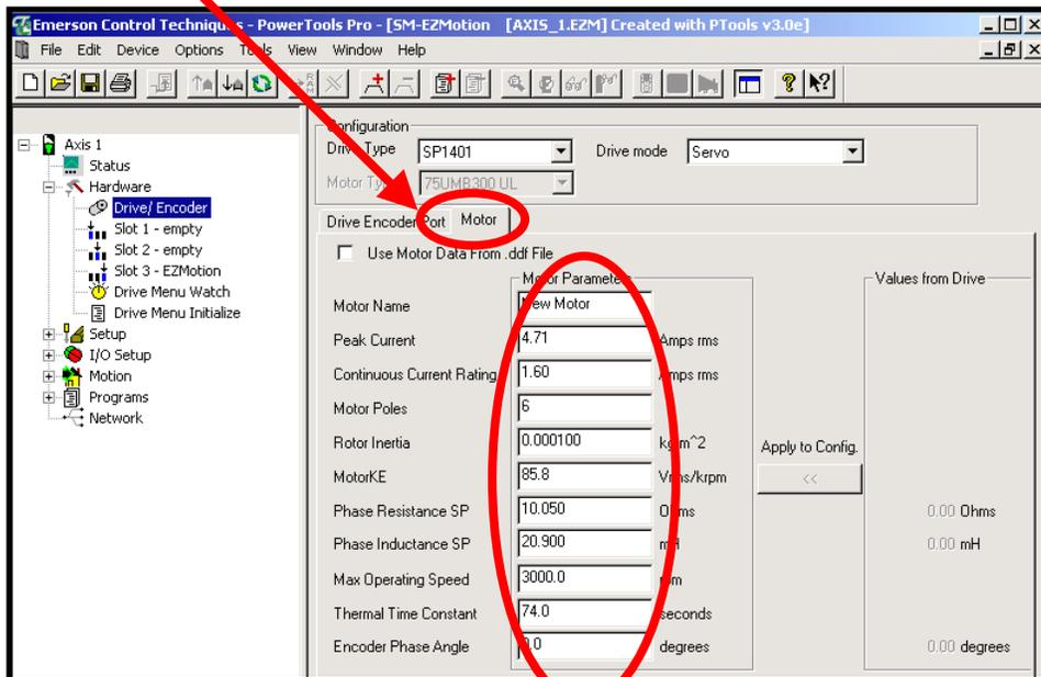
Enter motor data here. If you are unsure of the values to enter see the motor nameplate, refer to the data sheet or contact the motor manufacturer.
