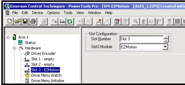
Choose the Slot with your EZMotion module and configure the Slot Number and Slot Module accordingly. Set up any other modules at this time.
